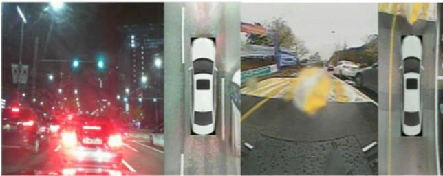
Fig. 2. Comparing front camera and AVM: left (heavy traffic condition) and right (rainy condition).
