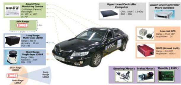
Fig. 3. Test vehicle configuration.
